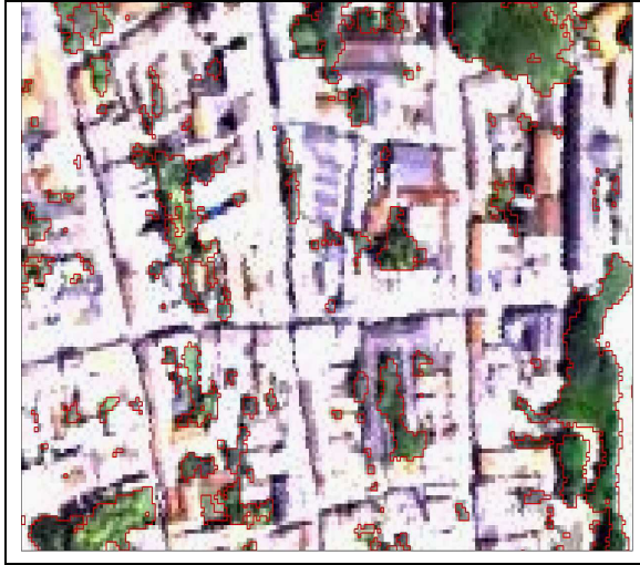
Fig. 4. Sample output of the automated identification and contouring process of buildings and vegetation, done on 56-channel AISA hyperspectral VNIR data by use of a patented method, mutated by burn scar analysis (Ferrucci & Hirn, 2005). In these pixels, LiDAR elevation measurement are expected to be precise within the error estimate ( \pm 0.15\text{m} averaged over buildings and bare soils).
