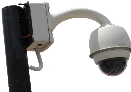
Fig. 2. A 0.4 mega pixel (PAL) Charge-Couple-Device CCD, internet surveillance camera used in this study is a Bosch's auto dome 300 series PTZ camera system
