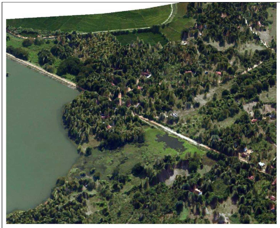
Fig. 2. Example of 3D rendering of combined LiDAR (1m planimetric resolution, 0.3 m precision in elevation on steady reflectors) and digital camera aerial scenery (resolution of 0.2 m). Picture taken over the artificial lake of Angunakolapelessa, north of Hambantota, south Sri Lanka.
