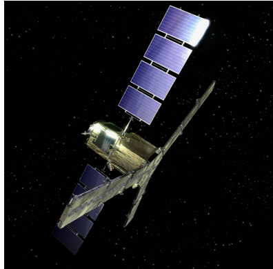
Fig. 9. Y-shaped antenna array of MIRAS and SMOS spacecraft of ESA
