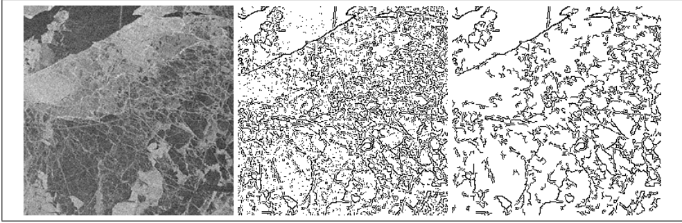
Fig. 4. A part of a SAR image ( \approx 25 \times 25 km, left), detected edges (middle) and the corresponding structured edges (right), i.e. edges which are parts of larger edge segments than a given threshold, here 10.
